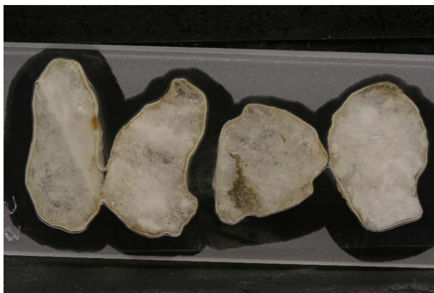
Figure 5 - Select drill chips with spodumene identified (height of slide ~26mm) (ASX Release 2 March 2018)
