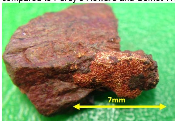
Figure 3 Gold nugget and fine "halo" gold in rock specimen ( ASX Release 19 March 2018 )
