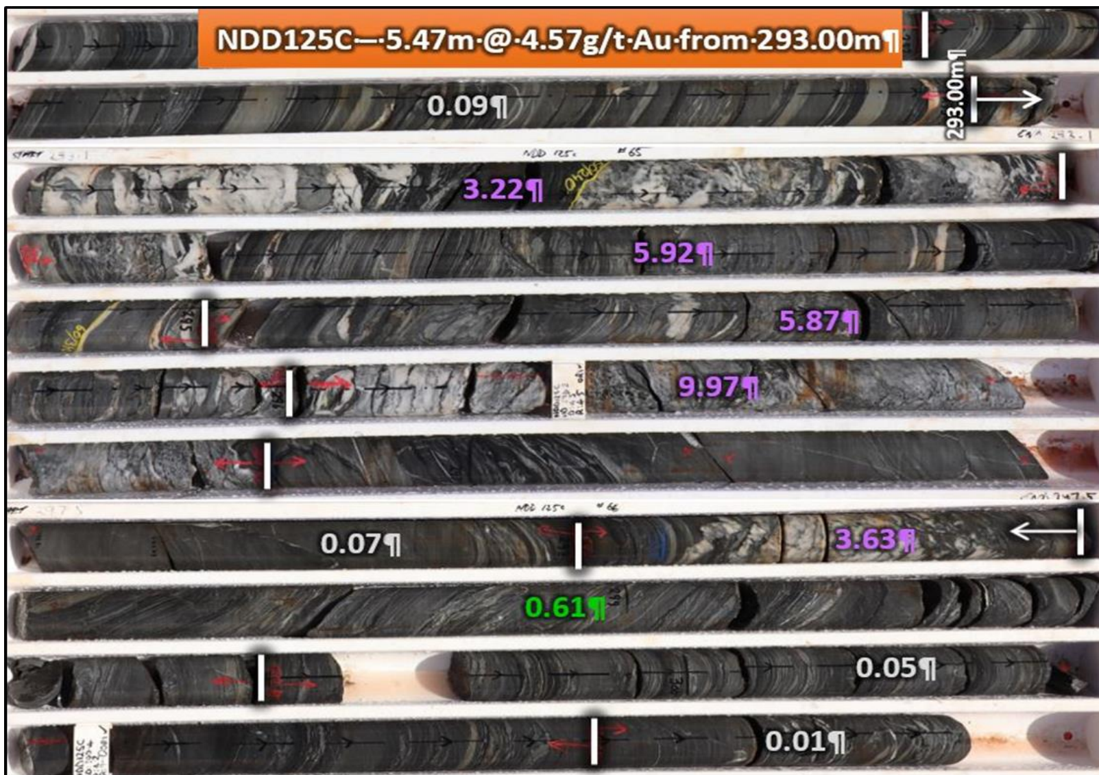
Figure 6 Withnell – Lode 1 mineralisation in drill core
