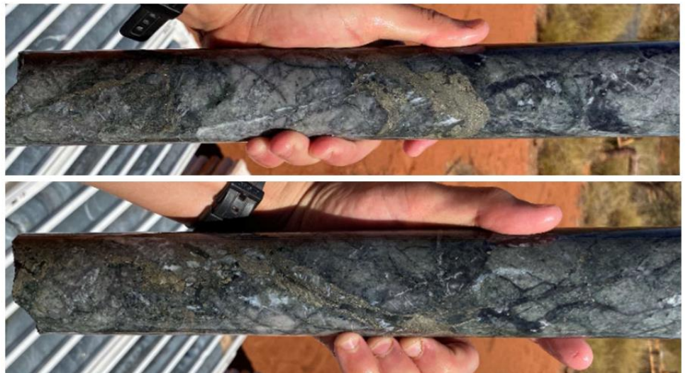
Figure 3. Diamond drill core from hole HERC233D (shown in Figure 2 above, labelled assays pending). The strong sulphide rich alteration and brecciation is similar to mineralisation in the Aquila Zone.
