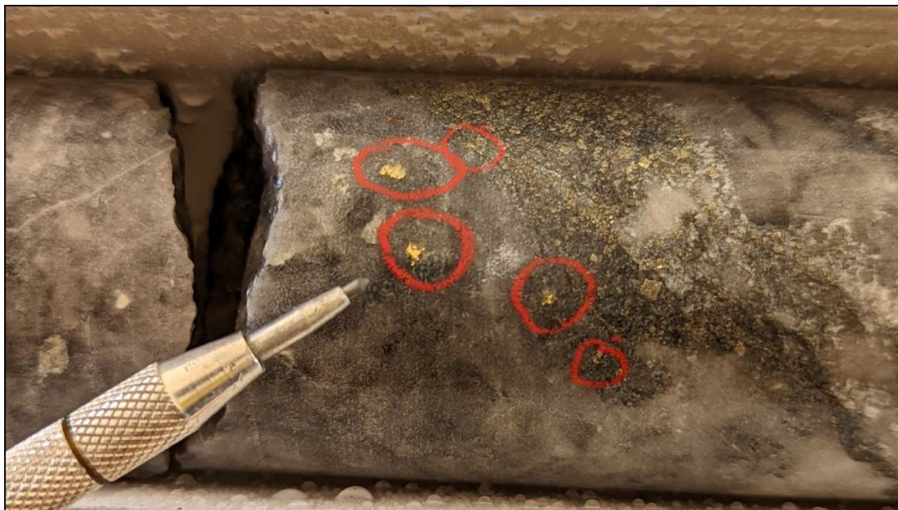
Figure 4 Visible gold in smokey quartz vein at 741m in HEDD136
